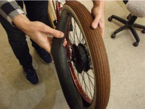
Now carefully remove the rear tire and inner tube. Pull them off to the "chain side".
